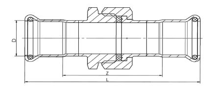
GDPRESS fittings offer reliable and consistent performance, combined with an easy installation process using common M-contour design and tooling compatability.
